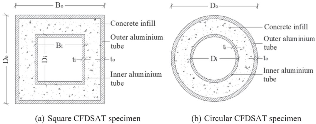
**Fig. 1.** Geometry of typical cross-sections of CFDSAT specimens.
