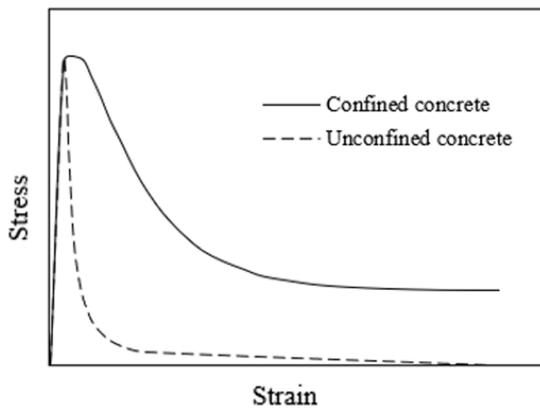
Fig. 9. Compressive response of confined concrete [52].
