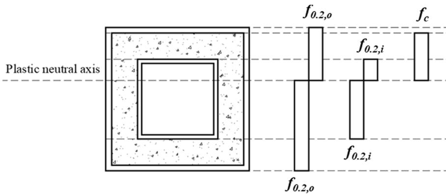
Fig. 20. Plastic stress distribution of a CFDSAT section.
