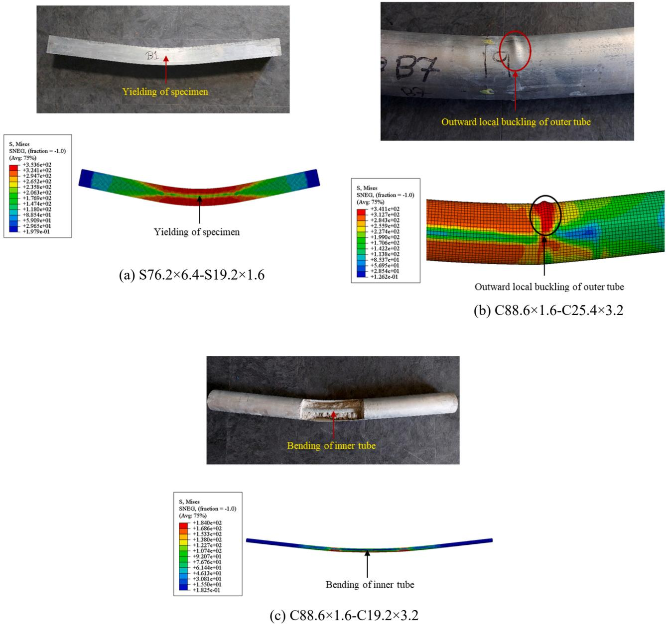
Fig. 12. Comparison of test and FE failure modes.
