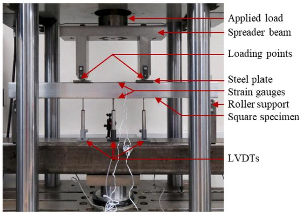
(a) Square CFDSAT specimen test set-up
