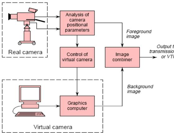
Fig 1 Camera tracking system for virtual studio
