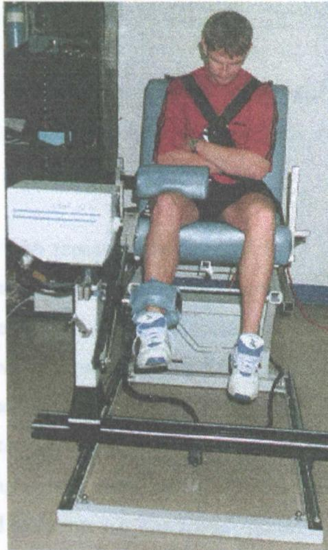
**Plate 3.2.1.** The isokinetic dynamometer (Lido Active<sup>®</sup>, Loredan, Davis CA) measuring dynamic strength of the knee extensors and flexors
