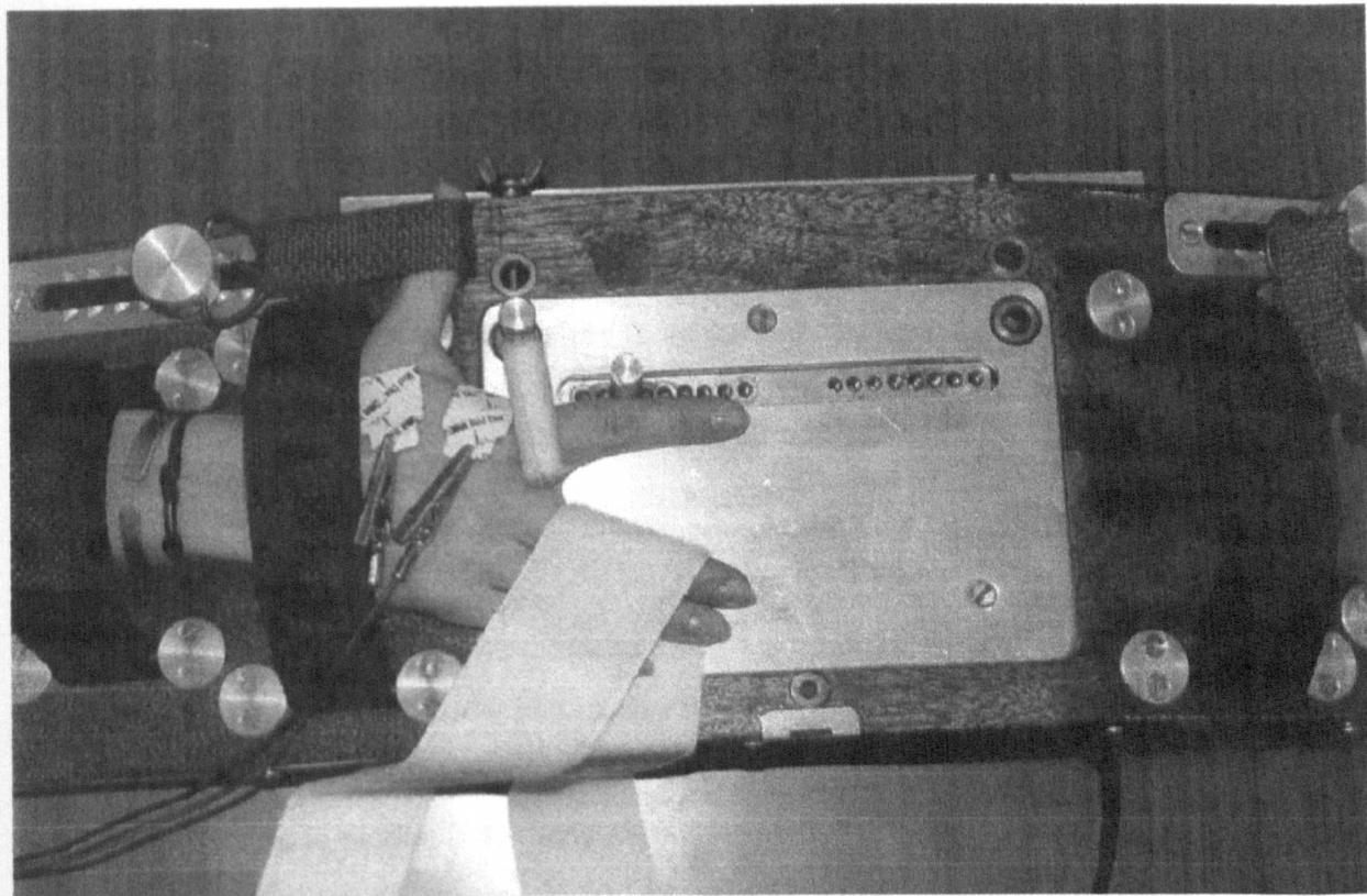
**Plate 3.5.1.** Dynamometer showing the index finger in relation to 1] force transducer 2] electrodes and 3] thumb
